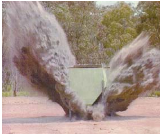
Rys. 9. Badania odporności nowego nadwozia firmy Timoney's na wybuch ładunku [7] Fig. 9. Timoney's innovative vehicle designs incorporate blast deflecting hulls, blow-away components and multiple floors [7]
